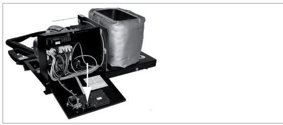
Figure 8.3/3 Position of back-up battery
