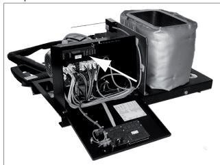
Figure 8.4/1: Position of power section
