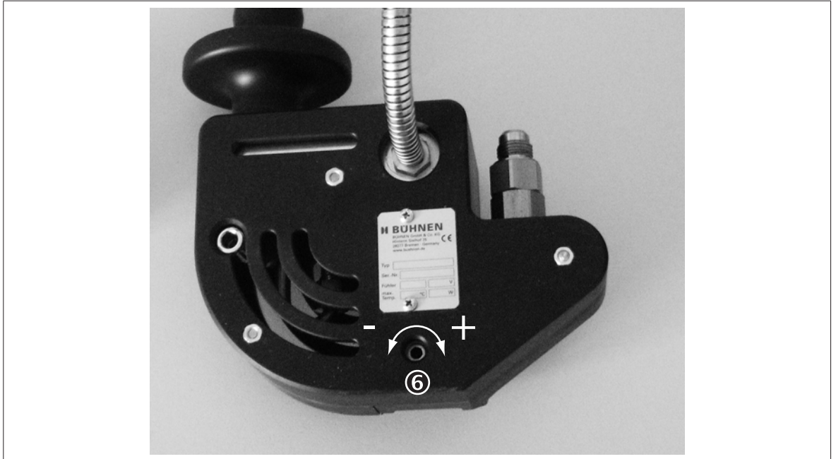
Figure 7: Setting the spray air
