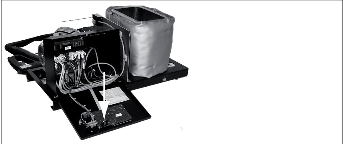
Figure 8.3/3 Position of back-up battery
